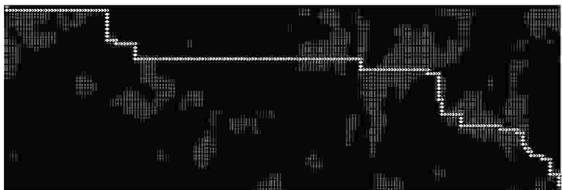
Fig. 3.14. Weighted terrain-based grid graph with a dimension of 50 \times 200 nodes (squares). Colour represents value of criterion c_2 : the colour of the node (square) describes the ability to camouflage: the darker the colour the smaller the ability to camouflage. The white colour describes the optimal path from the left-top to the right-bottom corner
